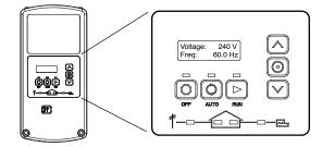
The RDC2 controller provides integrated control for the generator set, Kohler<sup>®</sup> Model RXT transfer switch, programmable interface module (PIM), and load management device.
